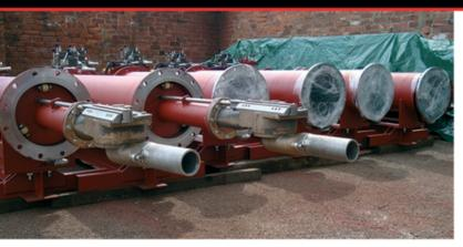
The Live Mastir Cannons are available as a contracted service for the desludging of crude oil storage tanks without man entry.
